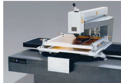
StencilLaser SL 600x600 from 1995
