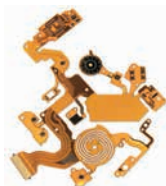
Full flexibility: precise, complex contour cutting and perfectly drilled holes with LPKF laser tech
